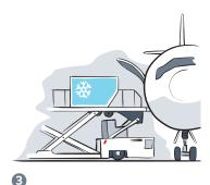
**Specialized cooling containers** ensure a temperature controlled transport on the apron and during loading.
